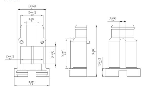
The tube lock are 2 parts, which hold the plug and RIC tube in place. They are kept together by a plug cover, which Sonion can customize to match specific BTE geometry
