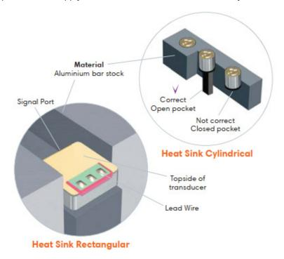
An alternative way to dissipate the heat from the transducers is to use a metal double sided tape on a metal block, provided that the sound outlet is not closed during the soldering. We recommend using this only if there are no alternative options and it should be done by experienced operators.
