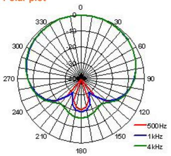
Note: when tubing is applied the polar responses and sensitivity of the directional microphone will change according to the new port spacing
